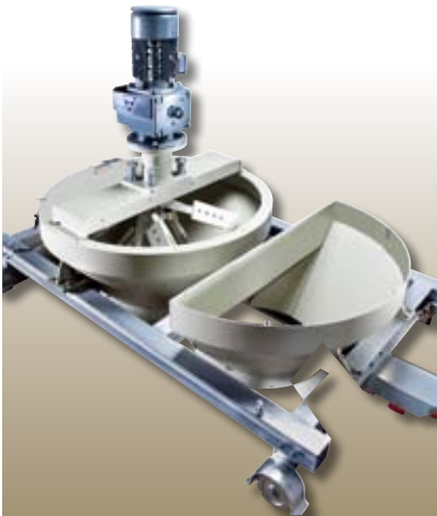
Travelling Continuous Flow Mixer with Single-Product Chute and HARDOX 400
