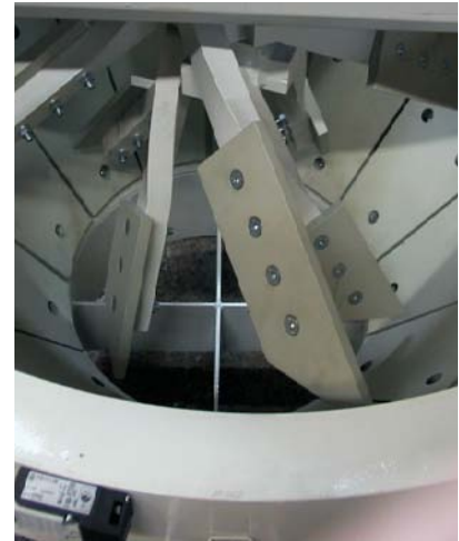
Cast iron tiles for mixer wall made of highly wear-resistant G-X350 CrMoNi 2021/25 mm (approx. 0.98 inches).
